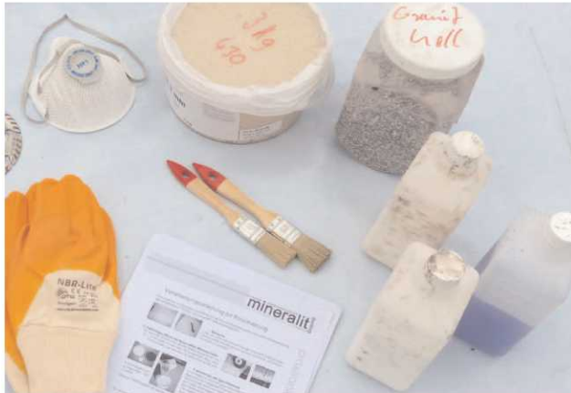
Masterbatch quartz sands (3 kg) , acrylate bond MMA G12-20 (blue), hardener Pergan 50 W (white powder)
